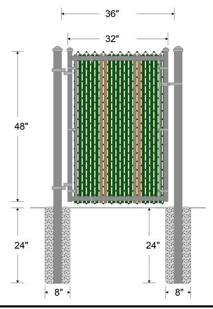
48" tall Chainlink Fabric with Knuckle / Knuckle Selvage and 2" Mesh Size.
